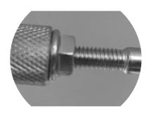
Please note – The locking nut behind the spigot must be loosened before adjusting. Turn the spigot clockwise to expose more thread, making sure its not being attached to the lever at this stage
