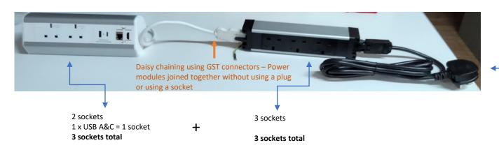
This plug will power both modules (2-meter power lead) = 6 Sockets
