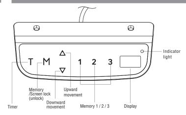
Note: If the control panel is used for the first time, please reset the system before any normal operation.
